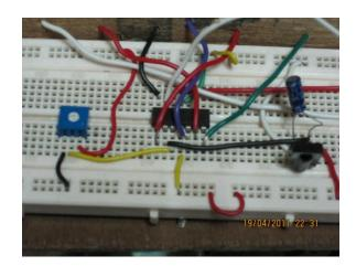
Fig 7.A picture of our IR receiver circuit
