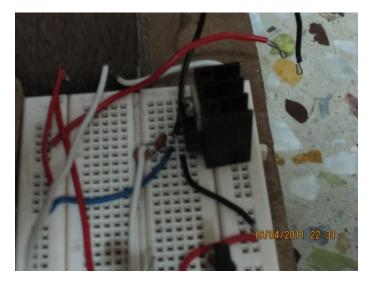
Fig13. A Photograph of the voltage supply block of the circuit. The large black structure is the7805 voltage regulator plotted with the heat sink. The red wire with the bare end is to be connected to ground while the black one is to be connected to 12V supply from an SMPS.
