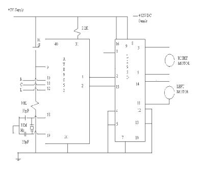
Fig 6.Microcontroller and driver circuit
